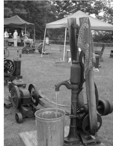
This water pump from the Maybie farm has been adapted to run by belt and could easily water the 125-head dairy herd.
